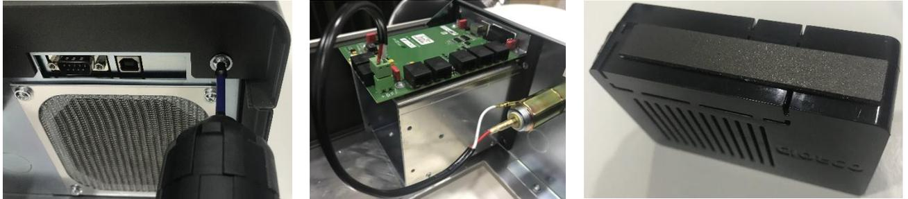
Use the magnetic strip to attach the E-Maxx to the inverter or near the inverter. Ensure that connection ports of the E-Maxx are accessible.
