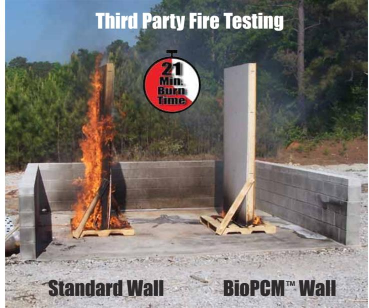
BioPCM™ is manufactured with your protection in mind, with a fire suppression element integrated to provide peace of mind. The fire testing photo above shows the condition of a timber construction walls after a period of 21 minutes.
